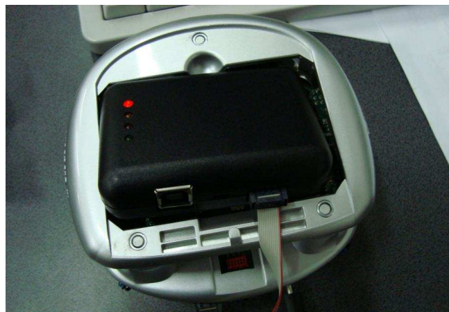
Figura 2.16: b) Kephera III + KoreConnect
