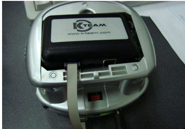
Figura 2.15: a) Kephera III + KoreConnect
